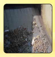
The Static Screen unit's unique bi-wave wedgewire screen panel, with double downward curves, increases the Coanda effect by rapidly stripping liquid from the influent as it hits the top of the screen panel. The rapid shearing maximizes solids capture and minimizes screen blinding.
